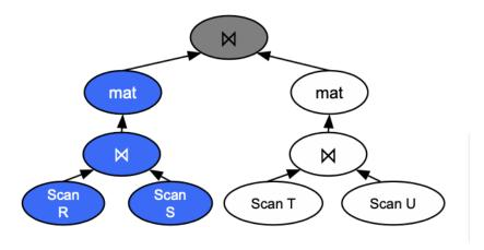
In bushy tree parallelism, the left branch and right branch can execute at the same time. For instance, scanning R, S, T, U can all happen at the same time. After that, joining R with S and joining T with U can happen in parallel as well.
