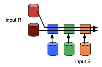
For instance, if relation R is small, we could do a broadcast join by sending R to all machines that have a partition of S. We perform a local join at each machine and union the results.
