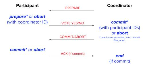
The asterisk \* in the diagram above means that the node must wait for that log record to flush to disk before sending the next message. Notice that in the presumed abort optimization,
