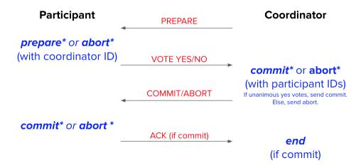
The asterisk \* in the diagram above means that the node must wait for that log record to flush to disk before sending the next message.
